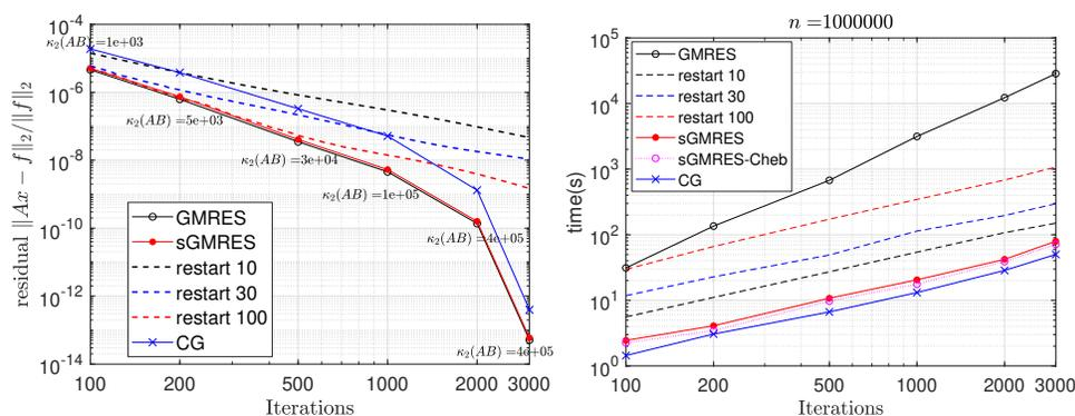
FIG. 3. *sGMRES versus GMRES: Laplacian system.* For a 2D Laplacian system  $\mathbf{Ax} = \mathbf{f}$  with dimension  $n = 10^6$ , these panels compare the performance of MATLAB `gmres` (with and without restarting) against the *sGMRES* algorithm (with 2-partial orthogonalization or the Chebyshev basis). Left: Relative residual and condition number  $\kappa_2(\mathbf{AB})$  of the reduced matrix associated with the  $k$ -truncated Arnoldi basis. Right: Total runtime including basis generation.
